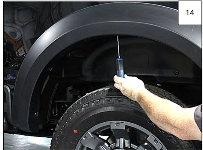
While holding flare to vehicle, start supplied Truss-Head Screws through the 4 topmost mounting holes in flare and into clips installed in Step 13. Apply pressure to flare towards vehicle body at each fastening point and tighten all fasteners.
