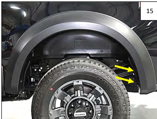
Install 2 supplied Plastic Retainers through flare and into factory holes at rear of wheel well.
