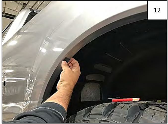
Peel liner from a supplied Foam Tab and center tab over each mark made in Step 10, folding each tab over the wheel well lip.
