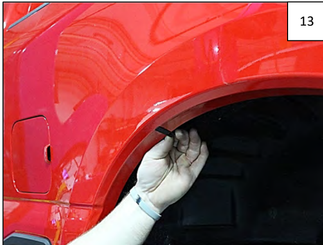
Slide a supplied Long "U" Clip over each foam tab, making edge of clip flush with outer edge of wheel well lip as shown.
