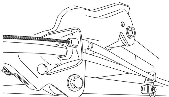
**1500 RAM ONLY.** Attach brake cable guide to supplied Brake Cable Bracket (31) and mount bracket with supplied hardware. Reattach brake cable and readjust brake cable adjustment nut to
