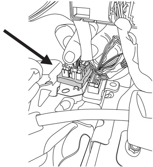
**Note: It's best to reach from both sides when installing 2 pin plug. Any open port on green plug can be used.**
