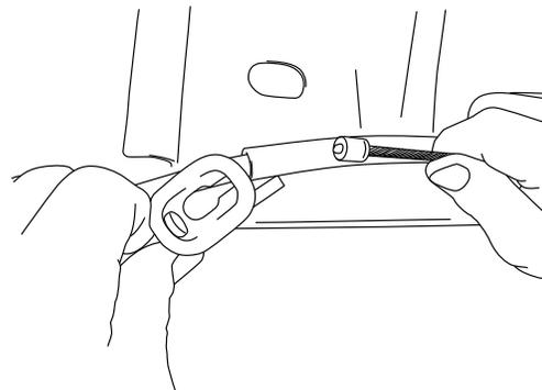
**1500 RAM ONLY.** Remove brake cable guide from frame by depressing locking tabs and sliding guide out through hole. Unthread brake cable from frame mount.
