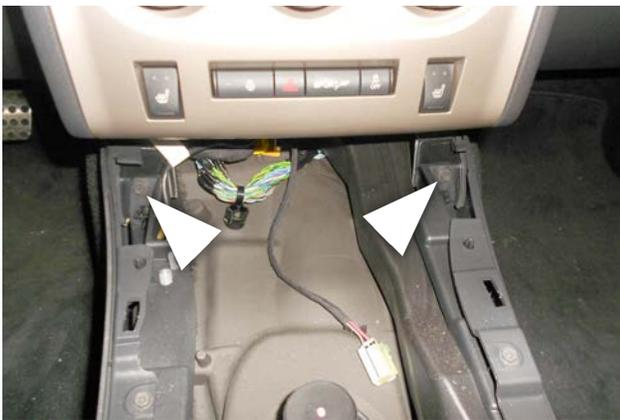
7. Remove the 2 screws at the front of the center console base.
