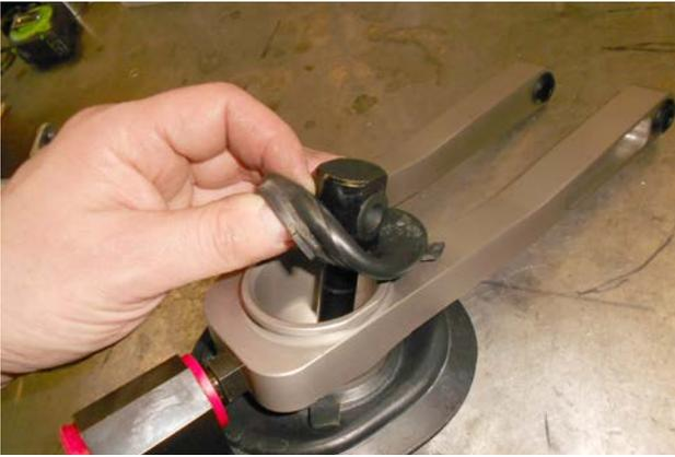
31. Pull the lower seal over the bottom of the shifter assembly. Fit the seal lip into its groove on the shifter.
