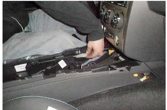
9. Remove the electrical connector located in the left side of the console.
