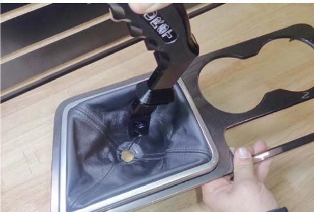
59. With the boot still inverted, insert the shift handle through the boot opening, with the front of the shift handle (finger grooves) pointing forward.
