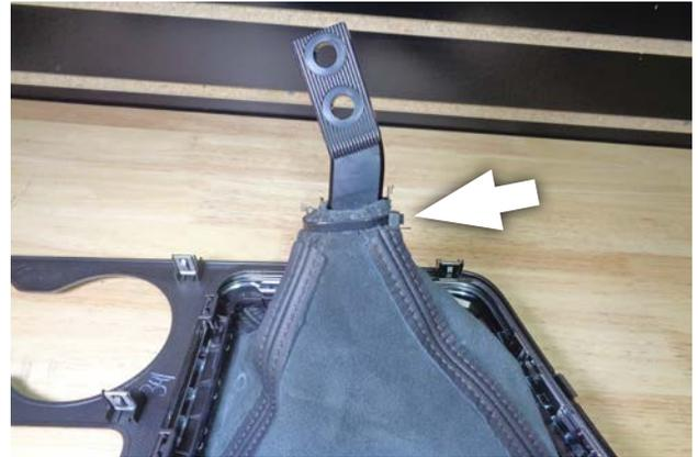
60. Use the **zip tie (9)** to secure the boot to the boot support. Start by engaging the zip tie to just the first "click." Then slip it over the boot until it is aligned with the groove in the boot support. Gradually tighten the zip tie, working it into the groove as you go. When the zip tie is fully tightened, trim off the tail.
