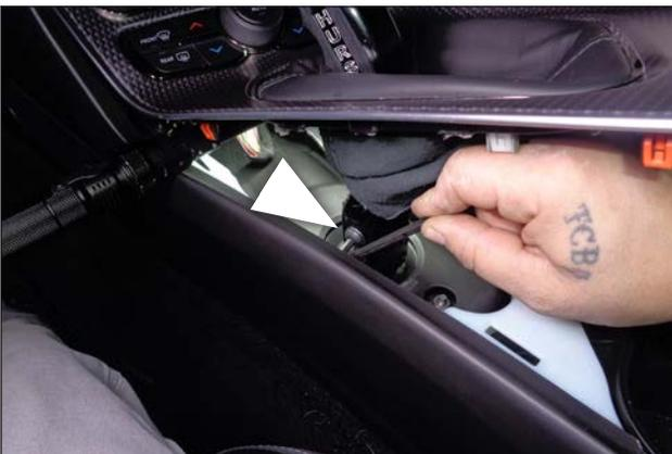
68. Fasten the shift handle to the **LEFT (driver) side** of the shifter block using **two 3/4"-long screws (5)** with thread-locking fluid, and **two lock washers (4)**.
