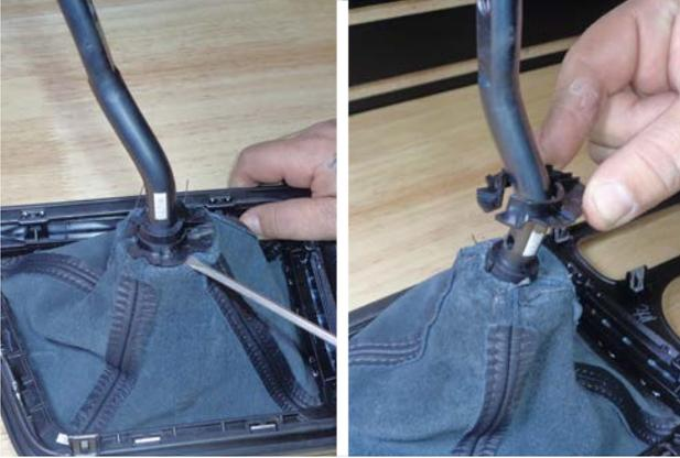
57. Turn the boot inside out. Carefully remove the plastic locking ring from the shift handle, then remove the handle from the boot.
