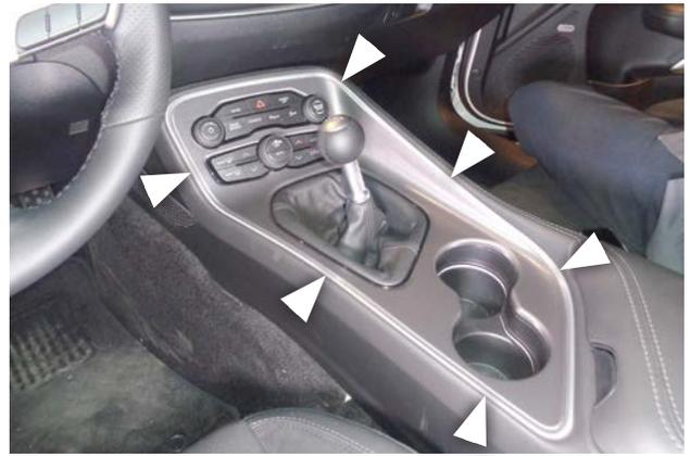
13. Use a trim removal tool to carefully separate the console bezel from the console.
