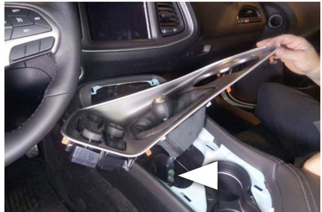
55. Hold the assembled console bezel, boot, and stick above the console, and insert the stick in the slot on the rear of the shifter. Install the 2 OEM screws with thread-locking fluid, and tighten them to 20 lb-ft torque.
