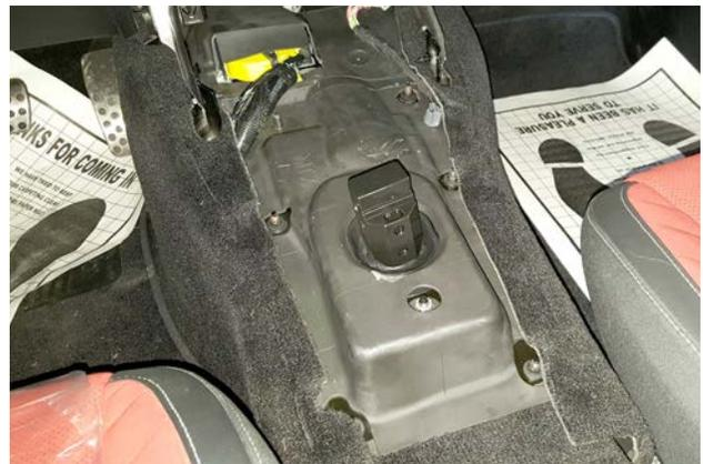
39. Lower the dust boot over the tunnel cover, and tuck it under the edges of the carpet.
