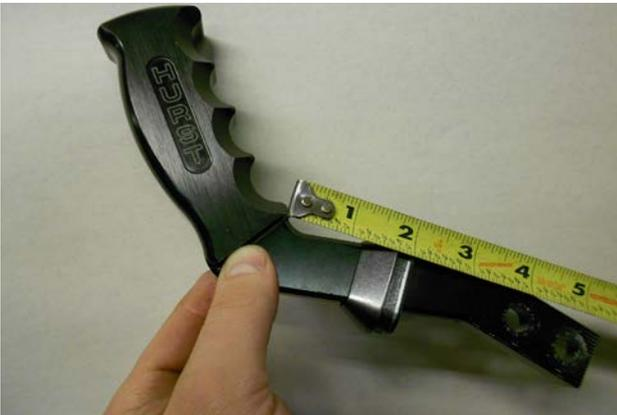
58. Slip the **boot support (8)** onto the **shift handle (3)** with the set screw hole facing rearward (away from the finger grooves). Install the **set screw (7)**, and tighten it with the boot support about 1-1/4" from the bottom of the grip.
