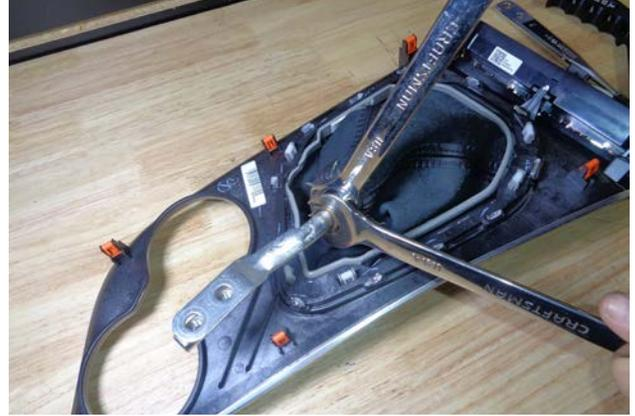
63. Turn the console bezel and boot upside down, and use 2 wrenches to loosen the shift handle jam nut.
