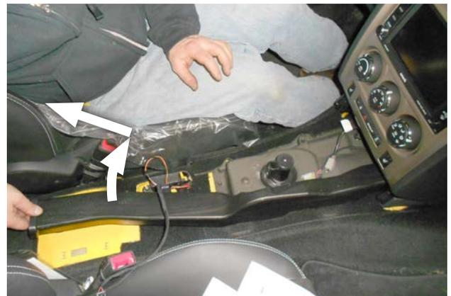
11. Lift the rear of the vent duct up sharply to release it. Then move the duct rearward to disengage its front end, and remove it from the vehicle.
