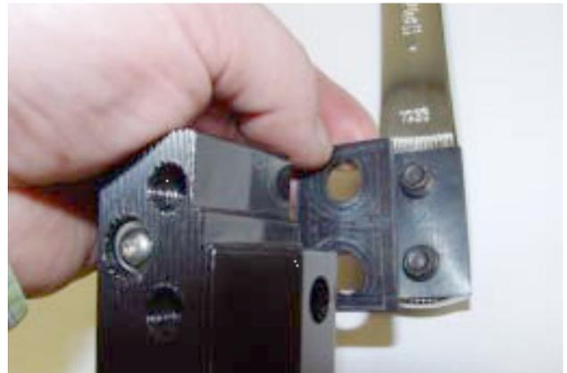
71. Reinstall the handle on the shifter block using the **two neoprene isolators (2)**, the **two 1"-long screws (6)** with thread-locking fluid, and **two NEW lock washers (4)**. (Do not reuse the previous lock washers.) Then reassemble shift boot and console bezel.
