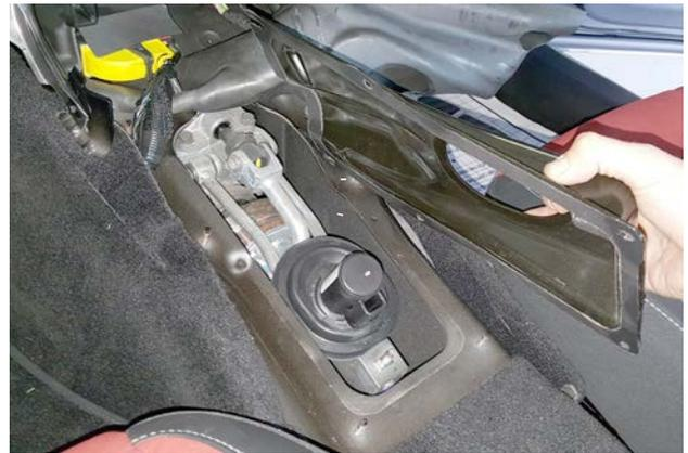
24. Remove the tunnel cover from the vehicle.
