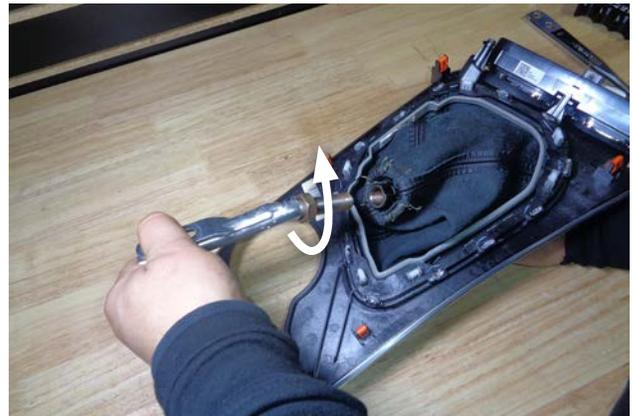
64. Unthread the stick and jam nut from the handle.
