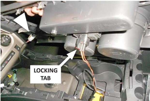
6. Remove the electrical connectors at the 12 volt outlet and the cup holder light. (Pull the red tab at the cup holder to unlock the connector.) Then remove the console cover from the vehicle.
