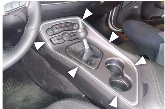
56. Snap the console bezel into the console.
