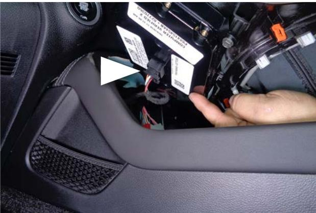
54. Reconnect the electrical wiring to the back of the control panel.
