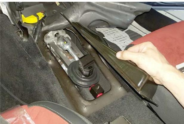
37. Reinstall the tunnel cover. Hand-start the 7 cover nuts, then tighten them to 15 lb-ft torque.
