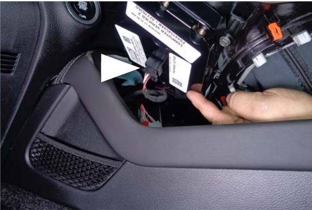
67. Move the assembled console bezel and shift handle into the vehicle, and reconnect the electrical wiring to the back of the control panel.
