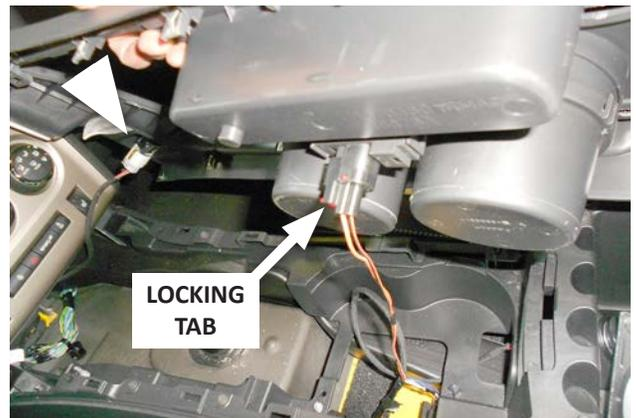
45. Return the console cover to the vehicle, and reconnect the wires to the 12 volt outlet and the cup holder light. Lock the cup holder light connector by pushing the red tab closed.
