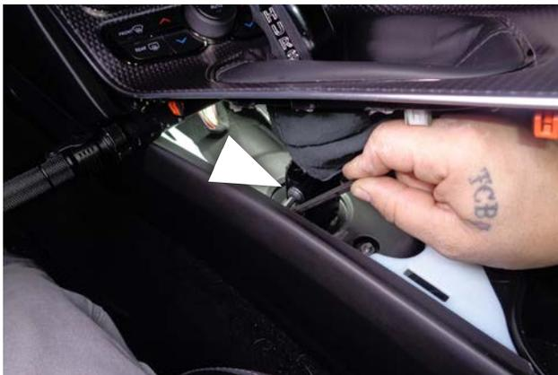
70. Remove the console bezel as required to access and remove the 2 shift handle screws.
