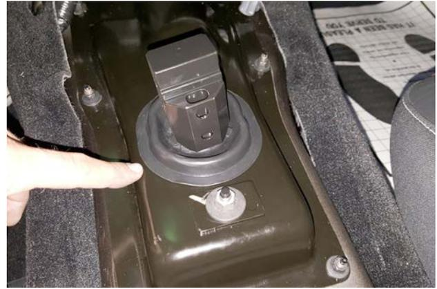
38. Secure the upper shifter seal to the tunnel cover by pulling its top flange up through the tunnel cover opening.
