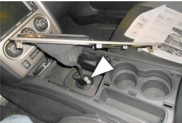
47. Hold the assembled trim bezel, boot, and stick above the console cover, and insert the stick in the slot on the rear of the shifter. Install the 2 OEM screws with thread-locking fluid, then tighten them to 20 lb-ft torque.
