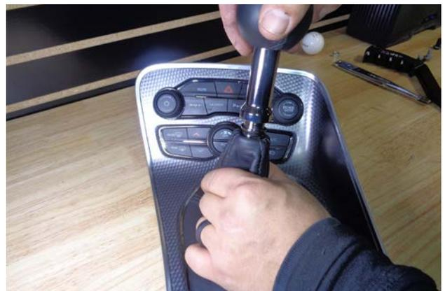
65. Carefully separate the elastic boot opening from the bottom of the shifter handle.
