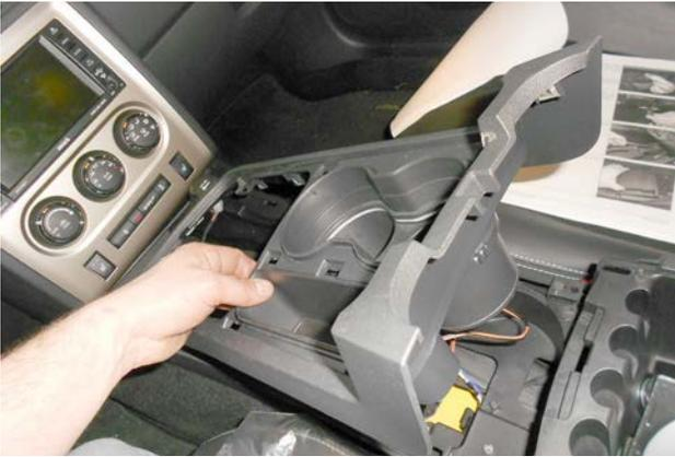
46. Snap the console cover into the center console.
