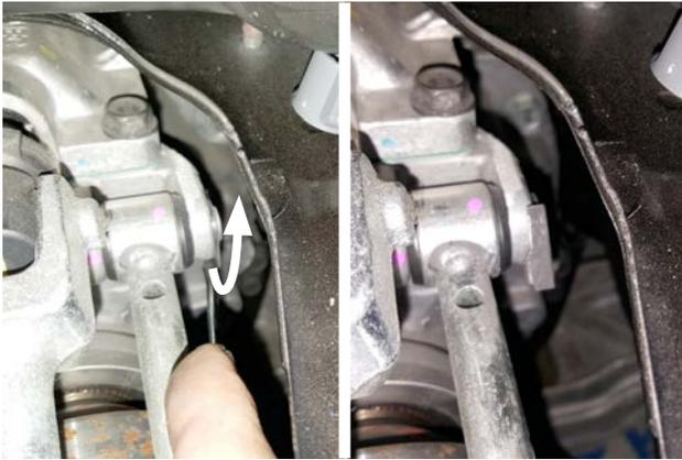
**NOTE:** A small screwdriver or dental pick may be necessary to rotate the locking tabs.
