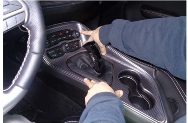
69. Snap the console bezel into the console.
