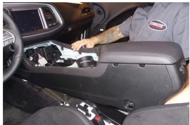
51. Carefully return the center console to the vehicle and place it in its final location. Be sure that the rear of the vent duct mates correctly with the opening at the rear of the console.
