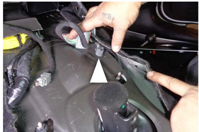
49. Push the harness clamp onto its button on the dust boot.
