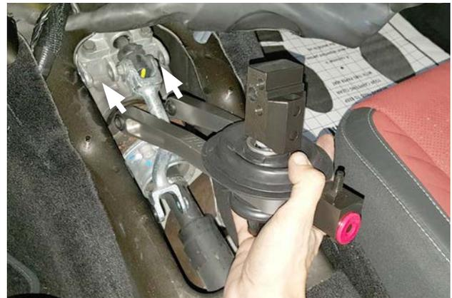
33. Insert the ends of the shifter yoke into their respective clevis ears on the transmission.
