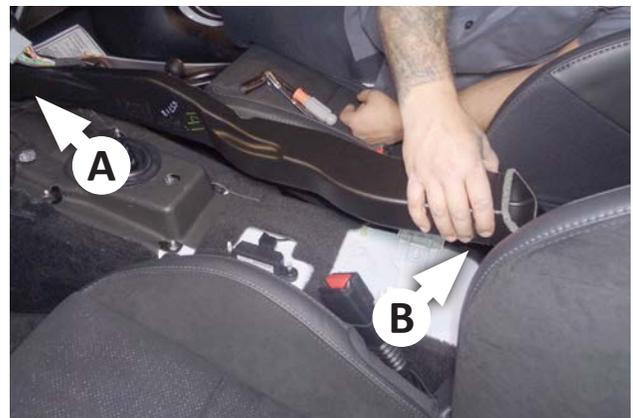
50. Insert the front of the vent duct into its opening (A) under the control panel, and snap it into place at the rear (B).
