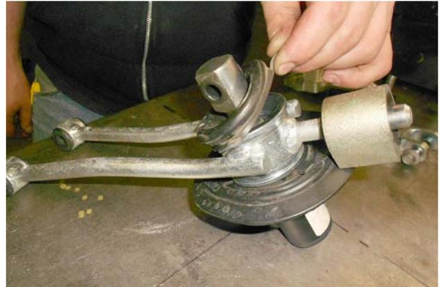
28. Remove the lower shifter seal.
