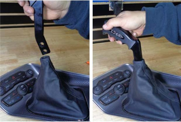
66. Insert the **shift handle (3)** through the boot, and push the boot opening up the handle.
