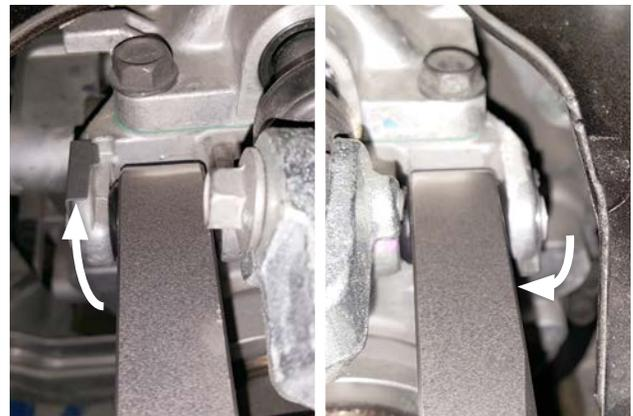
34. Insert the 2 locking pins with the lock-tab flats facing rearward, then rotate the lock-tabs 1/4 turn counter-clockwise (left tab to the top, right tab to the bottom).
