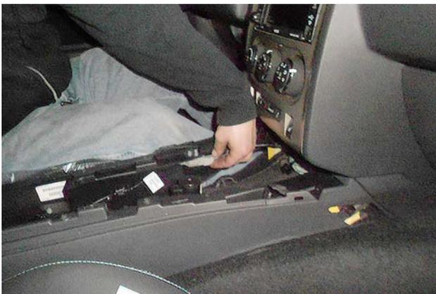
42. Rotate the console to upright and put it in its final location. Be sure that the rear of the vent duct mates correctly with the opening at the rear of the console. Then reconnect the wires in the left side of the console.
