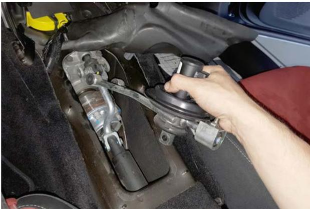
27. Remove the shifter assembly from the vehicle.
