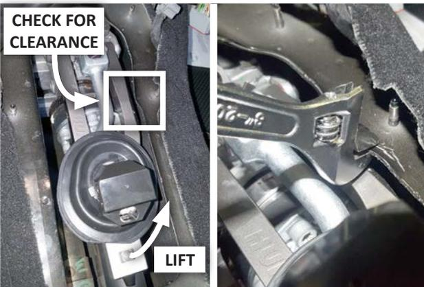
36. Lift the rear of the yoke to the approximate height it will come to once the tunnel cover is installed, then check for sufficient clearance between the yoke and the transmission tunnel. If necessary, bend the edge of the tunnel upward with an adjustable wrench to ensure sufficient clearance.
