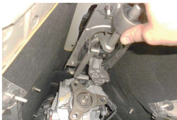
34. Reinstall shifter housing.
