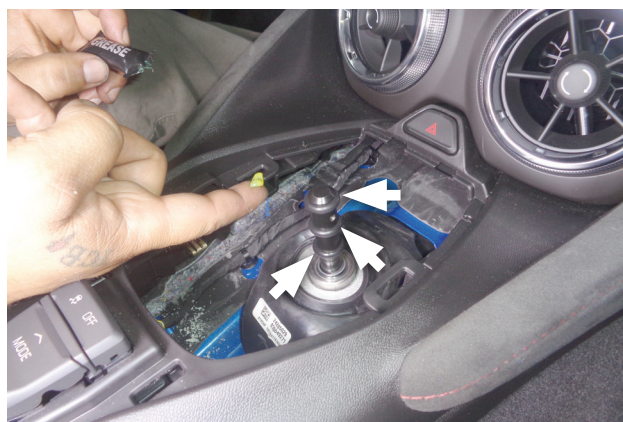
36. Grease (x3) o-rings on shift lever.
