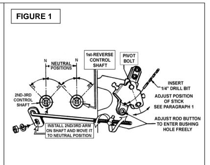
2. Install the  $2^{nd} - 3^{rd}$  arm on the transmission control shaft. Fasten the arm to the shaft with the stock hardware. Assembly the proper rod to the arm with a bushing and fasten with a spring clip. With bushings installed, rod adjusting buttons must be adjusted to fit freely into the holes in the levers. Fasten the button with a spring clip.
