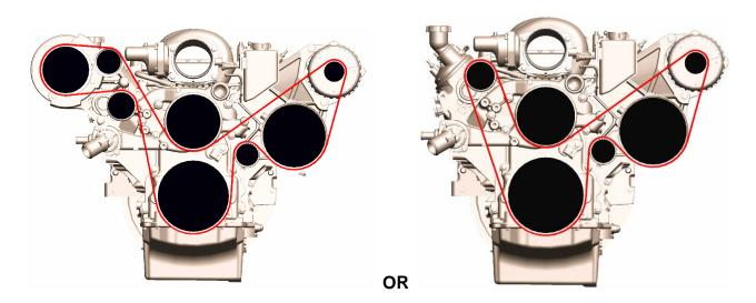
Both the bracket application and pulley diameters vary and will directly affect belt length. To acquire the measurement for the correct belt, perform the following:
