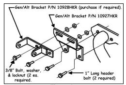
Figure A1-Stock Alternator Bracket
