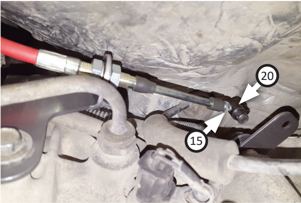
23. Thread nut (15) and cable pivot (20) onto cable, approximately to middle of threaded cable end.
