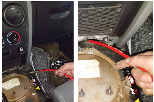
21. Route threaded end of cable down through entry point under center controls.
