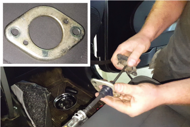
19. Separate shift cable seal plate from shift cable and retain it for later use.
