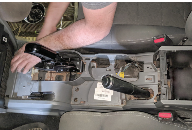
31. Install console case (removed step 6) using fasteners (x10) (step 5), then install console top (step 4). (As shown in following picture)
