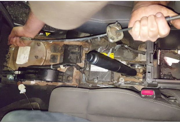
18. Move back into vehicle cab, then carefully pull factory shifter cable out through entry point under center controls.
