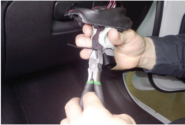
14. Trim the tail off the cable tie.
