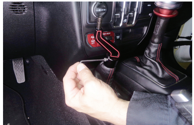
18. Apply medium strength thread locking fluid to cap screw (4) and install it in the shift handle.
