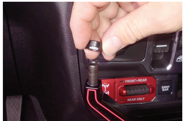
19. Run the jam nut (2) all the way down the knob screw, with the wrench flats facing down.
