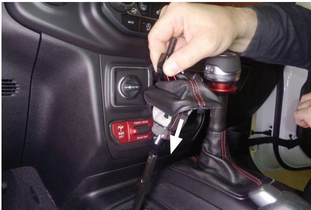
15. Install the shift handle and boot over the shift lever.
