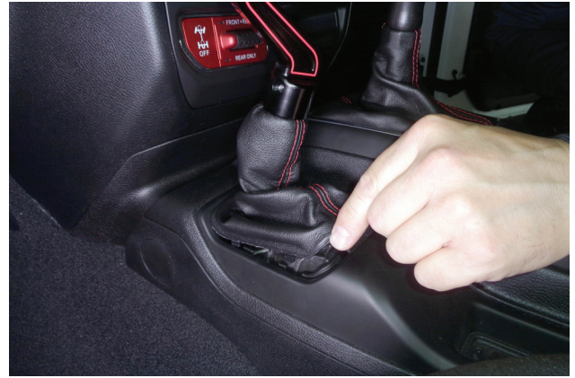
17. Pull the shift boot down and snap the boot frame into the center console.
