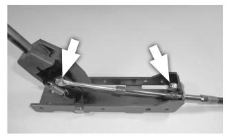
3. Assemble the shifter and cable. At the front (eye-end) of the cable, pull the two plastic dust boots all the way forward. Insert the cable through the notch in the shifter base. Secure the cable eye to the shifter pin with the E-clip. Then secure the cable housing tab to the shifter base with the 1/4-20 × 5/8" bolt and lock nut. Finally, push both plastic dust boots back over their respective joints.
