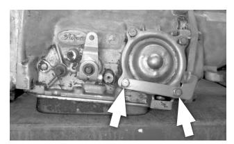
A. C4 / C5 transmissions: Install the cable bracket at the two lower servo cover bolt holes, using the two stock bolts. Tighten the bolts to 12-13 ft-lbs torque.
