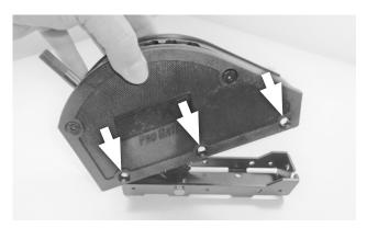
2. Disassemble the shifter: Remove the knob and jam nut from the shift lever. Remove the 6 countersunk screws from the bottom of the shifter (3 on each side). Then remove the gate plate and side cover assembly from the shifter base.
