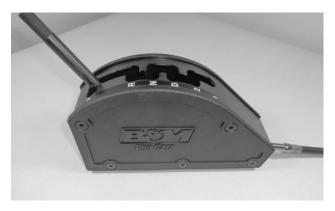
**10.** Ensure there is no debris in the shifter mechanism, then reinstall the assembled gate plate and side covers on the shifter base (3 screws on each side).
