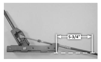
6. **Drill the cable hole.** Mark the center for the shifter cable hole 5-3/4" from the rear bend of the left shifter base. Move the shifter and cable out of the way, and drill or cut a 2" diameter cable hole through the floor.
