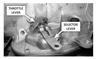
**13. Disconnect stock controls:** Loosen the throttle lever pinch bolt, remove the lever from its shaft, and carefully move the lever and linkage aside, allowing them to hang free. Remove and discard the stock selector lever and shift linkage.
