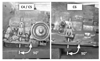
With the selector shaft still in DRIVE, align the selector lever perpendicular to the oil pan split-line, then tighten the fasteners. The lever should travel smoothly back and forth, with a positive "click" in each detent.
