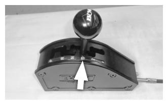
A. With the selector lever still in DRIVE (from Steps 25 and 26) and the shifter in the DRIVE position (shown), adjust the cable bracket nuts (and swivel, if necessary) until the swivel slips freely in and out of the selector lever hole.
