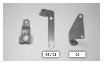
**22. Get the Ford selector lever and appropriate cable bracket** for your transmission from the parts kit.
