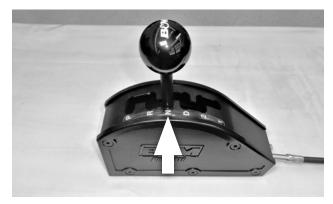
A. At the transmission, manually move the selector lever to the NEUTRAL detent (3 clicks back from full-forward, or FIRST). Then in the vehicle, move the shifter handle to NEUTRAL. Adjust the large cable bracket nuts until the swivel slips freely in and out of the selector lever hole.
