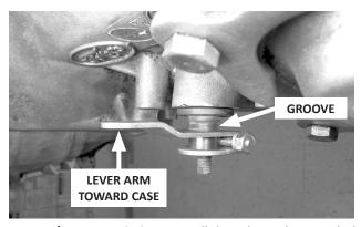
A. <u>C4 / C5 transmissions</u>: Install the selector lever with the lever arm **toward** the transmission case.
