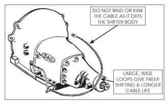
9. Route the cable approximately as shown. Avoid any sharp bends which may kink or otherwise damage the cable. Seal the cable hole shut to keep exhaust fumes, water, etc. out of the passenger compartment. Use clamps and/or cable ties (customer supplied) to secure the cable housing in such a way as to prevent contact with the exhaust system, engine, or any moving parts.
