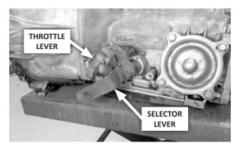
23. Disconnect stock controls: Remove and retain the nut and lock washer holding the throttle lever on its shaft. Carefully remove the throttle lever, and move it and its linkage aside, allowing them to hang free. Remove and discard the stock shift linkage.
