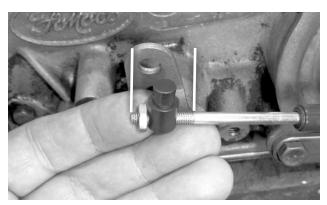
**29.** Thread the swivel onto the cable to about the middle of the threaded section, then reinstall (but do not yet tighten) the jam nut.
