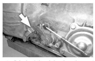
**33. Reinstall the throttle lever, lock washer and nut** on the throttle shaft and tighten securely. The throttle lever must operate smoothly with no binding.
