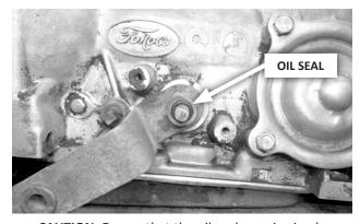
**CAUTION:** Ensure that the oil seal remains in place between the selector and throttle shafts. If the seal comes out, replace it before continuing.
