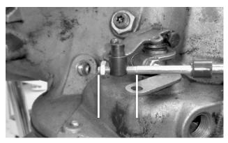
**17.** Thread the swivel onto the cable to about the middle of the threaded section, then reinstall (but do not yet tighten) the jam nut.
