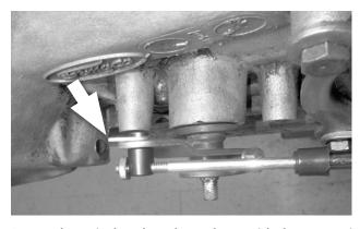
**32.** Secure the swivel to the selector lever with the cotter pin. Operate the shifter through all the gear positions, verifying that it operates correctly.
