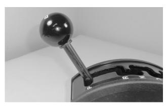
**11. Reinstall the jam nut (flats down) and shift knob.** Orient the knob as desired, then tighten the jam nut.
