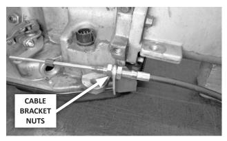
16. Attach the shifter cable to the cable bracket: First remove the small jam nut, both plastic dust boots, and one large nut and lock washer, from the cable. Then insert the cable through the cable bracket, reinstall the lock washer and nut (loosely, to allow room for adjustment), and reinstall the dust boots.
