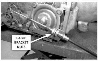
28. Attach the shifter cable to the cable bracket: First remove the small jam nut, both plastic dust boots, and one large nut and lock washer, from the cable. Then insert the cable through the cable bracket, reinstall the lock washer and nut (loosely, to allow room for adjustment), and reinstall the dust boots.
