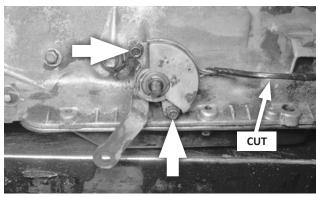
24. If your transmission is equipped with a neutral safety / backup light switch: Remove the two mount bolts and slide the switch off the selector shaft. Cut the wiring harness between the switch and its connector, and discard the switch. (If you install the B&M 80850 Pro Gate Switch Kit, the wires from the connector will be routed to the switches later.)
