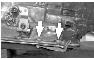
6. C6 transmissions: Install the cable bracket at the two left rear oil pan bolt holes, using the two 5/16-18 × 1" bolts and flat washers. For stamped sheet-metal (stock) pans, use the two spacers between the pan and bracket. (Spacers are not used with cast aluminum pans.) Tighten the bolts to 12-13 ft-lbs torque.
