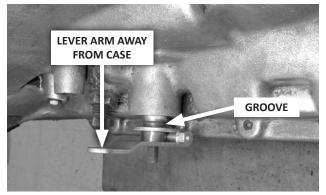
**B.** <u>C6 transmissions</u>: Install the selector lever with the lever arm **away from** the transmission case.
