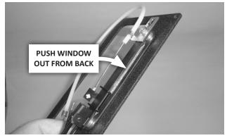
14. If you are using the shifter with a 4-speed transmission, replace the 3-speed indicator window in the cover assembly. From the underside of the cover, carefully push the 3-speed window out, and install the 4-speed window.
