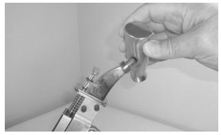
**15. Temporarily install** the **1/2-20 jam nut** and **T-handle** on the shifter, to permit easier shifting during installation. (The handle will be removed and reinstalled later.)
