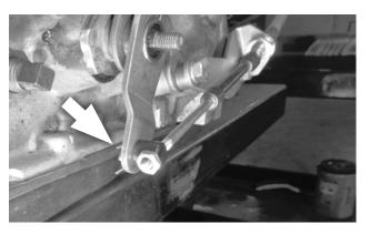
**35.** Secure the swivel to the selector lever with the cotter pin. Operate the shifter through all the gear positions, verifying that it operates correctly.
