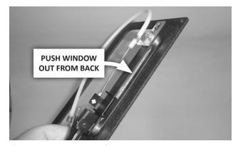
56. If you are using the shifter with a GM 4-speed transmission, replace the 3-speed indicator window in the cover assembly. From the underside of the cover, carefully push the 3-speed window out, and install the 4-speed window. (Use the 3-speed window for all other transmissions, including Chrysler and Ford 4-speeds.)
