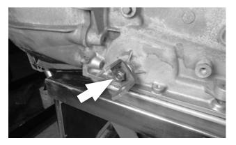
**41. Disconnect stock controls:** Remove and retain the selector lever nut. Remove and discard the selector lever and shift linkage.
