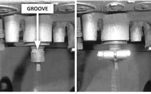
**NOTE:** If the selector shaft is grooved as shown, center the lever between the groove and the end of the shaft, so that the lever's inboard clamping surface does not land in the groove.
