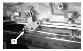
B. Adjust cable bracket nuts (and the swivel, if necessary) until the swivel slips freely in and out of hole "F" in the selector lever. Gradually tighten the cable nuts against the bracket while continuing to check the fit of the swivel in the selector lever.
