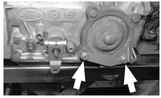
A. <u>C4 / C5 transmissions</u>: Install the <u>cable bracket</u> at the two lower servo cover bolt holes, using the two 5/16-18 × 1" bolts, flat washers and <u>spacers</u>. Tighten the bolts to 12-13 ft-lbs torque.
