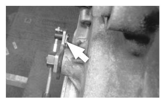
**49.** Secure the swivel to the selector lever with the cotter pin. Operate the shifter through all the gear positions, verifying that it operates correctly.
