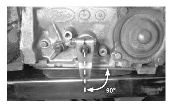
29. Install the B&M selector lever using the 1/4-20 × 1-1/2" bolt, lock washer and nut. (See NOTE on next page.) With the selector shaft still in NEUTRAL, align the selector lever perpendicular to the oil pan split-line, then tighten the fasteners.
