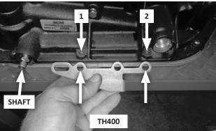
**43.** Check cable bracket fit: Remove the two oil pan bolts to the rear of the selector shaft. Determine which cable bracket holes will be used on your transmission.
