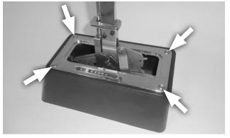
63. Secure the cover assembly to the tower with the four 3/4" self-tapping Phillips head screws.
