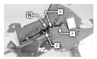
A. On the transmission, manually move the selector lever to the NEUTRAL detent (that is, 2 clicks back from full-forward / PARK). Then in the vehicle, move the shifter to the NEUTRAL position.
