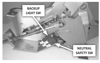
9. Install the two switches on the shifter mechanism as shown, using the two #4-40 × 1-1/4" screws, lock washers and nuts.
