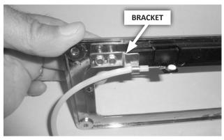
**58.** Run the shifter through all the gears to check indicator operation. If the indicator needs adjustment, loosen the 2 screws holding the cable bracket to the cover assembly, slide the bracket to adjust the indicator position, and re-tighten the screws carefully (they are threaded into plastic).
