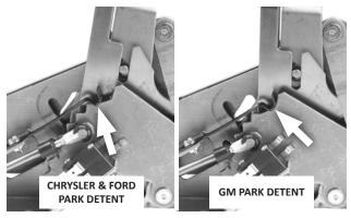
CAUTION: The shifter has two PARK positions — the first (lever full-forward) is for GM transmissions; and the second (one position back) is for Chryslers and Fords. To avoid stretching the shifter cable when shifting into PARK, NEVER force the shifter past the second (rear) PARK position (which corresponds to your transmission selector lever's PARK detent).
