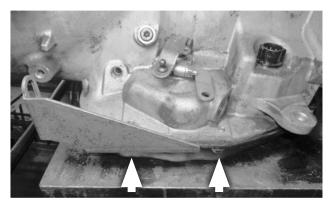
**15. Install the cable bracket** at the two pan bolt holes directly below the selector lever, using the two **5/16-18** × **1" bolts** and **flat washers.** For stamped sheet-metal (stock) pans, use the two **spacers** between the pan and bracket. (Spacers are not used with cast aluminum pans.) Tighten the bolts to **12-13** ft-lbs torque.
