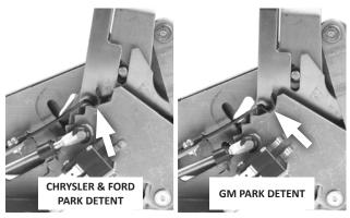
CAUTION: The shifter has two PARK positions — the first (lever full-forward) is for GM transmissions; and the second (one position back) is for Chryslers and Fords. To avoid stretching the shifter cable when shifting into PARK, NEVER force the shifter past the second (rear) PARK position (which corresponds to your transmission selector lever's PARK detent).
