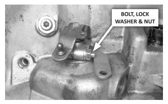
14. Install the B&M selector lever using the 1/4-20 × 1-1/2" bolt, and a 1/4" lock washer and nut. Be sure the lever is not pushed down against the transmission case, which could cause binding. The lever should travel smoothly back and forth, with a positive "click" in each detent. Then reinstall the throttle lever and linkage, tighten its pinch bolt securely, and check for smooth operation.
