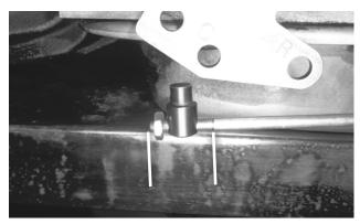
**46.** Thread the swivel onto the cable to about the middle of the threaded section, then reinstall (but do not yet tighten) the jam nut.
