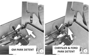
CAUTION: The shifter has two PARK positions — the first (lever full-forward) is for GM transmissions; and the second (one position back) is for Chryslers and Fords. Always push the lever FULLY FORWARD to put the transmission into PARK. Otherwise the transmission's park pawl will not engage, which will allow the vehicle to roll. See "Operation" for further information.
