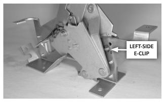
**7.** Configure the speed limiter pin for your application as shown below. (To remove the pin, remove the left-side e-clip, then push the pin out the right side.)
