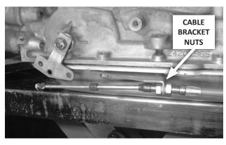
**45.** Attach the shifter cable to the cable bracket: First remove the small jam nut, both plastic dust boots, and one large nut and lock washer, from the cable. Then insert the cable through the cable bracket, reinstall the lock washer and nut (loosely, to allow room for adjustment), and reinstall the dust boots.
