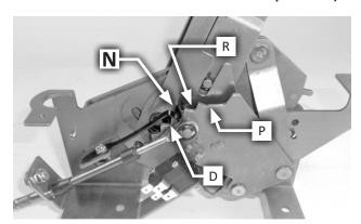
A. With the selector lever still in NEUTRAL (2 clicks from PARK), place the shifter in the NEUTRAL position, and adjust the cable bracket nuts (and swivel, if necessary) until the swivel slips freely in and out of the selector lever hole.
