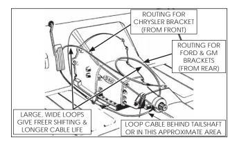
11. Route the cable approximately as shown, based on your application. Avoid any sharp bends which may kink or otherwise damage the cable. Seal the cable hole shut to keep exhaust fumes, water, etc. out of the passenger compartment. Use clamps and / or cable ties (customer supplied) to secure the cable housing in such a way as to prevent contact with the exhaust system, engine, or any moving parts.
