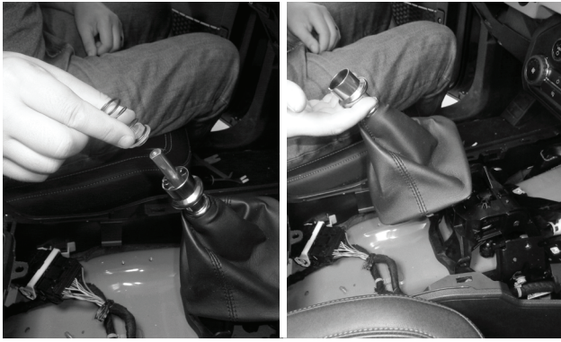
16. Remove the lockout spring and bushing, then remove the boot assembly.
