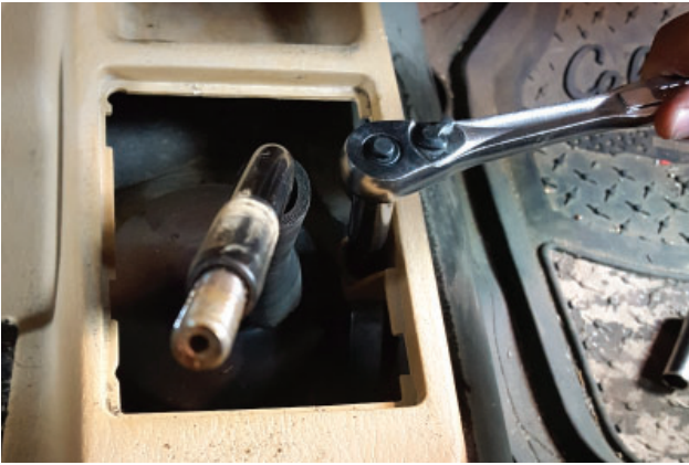
6. Remove and retain center console fastener near shifter.
