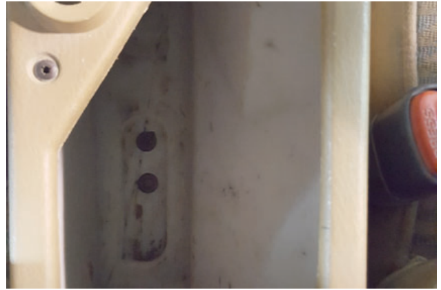
9. Remove and retain center console bolts (x2) from storage console.
