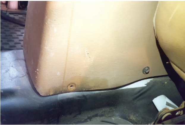
7. Remove and retain fasteners securing passenger side of center console.
