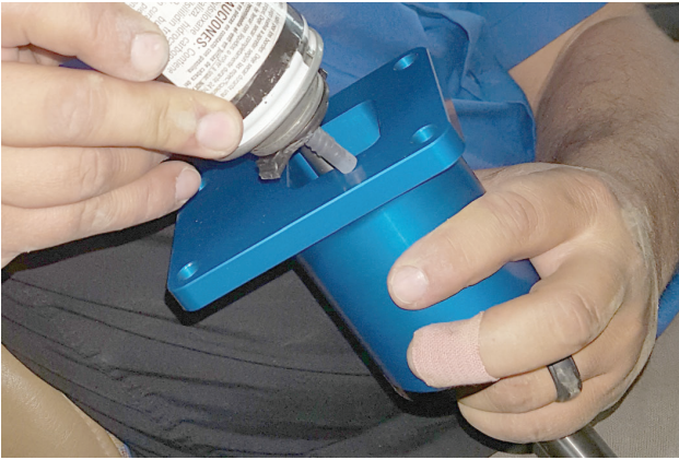
18. Install new shifter base gasket (not included) or apply RTV silicone sealant to the B&M shifter base.
