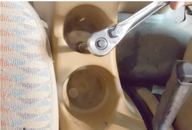
8. Remove and retain center console fasteners from cup holder.
