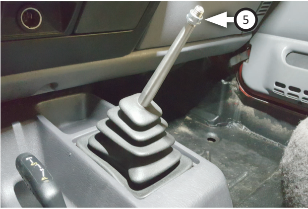
23. Re-install shift boot, then thread shift handle lock nut (5) onto shifter stem.
