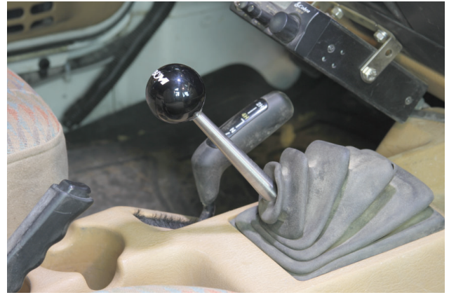
26. Test shifter engagement in each gear, then tighten all parts and verify shifter function once more.
