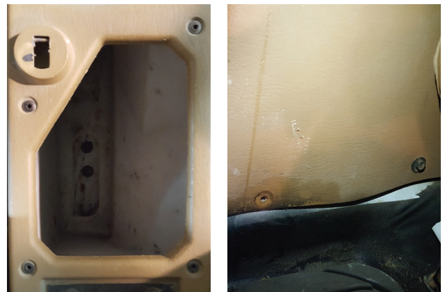
22. Set console cover back into place then secure it using fasteners from step 6 through 9.
