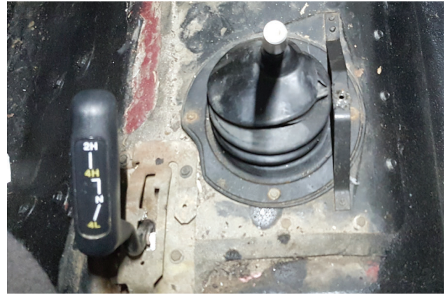
21. Re-install rubber protective boot and bolts removed step 12.
