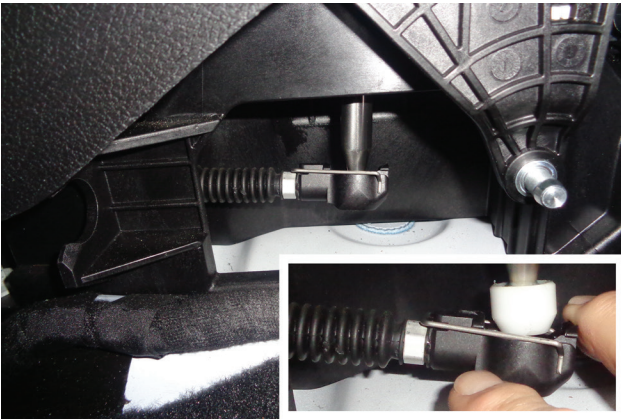
31. Install lower cable onto pivot cup, accessed from front passenger side of console.
