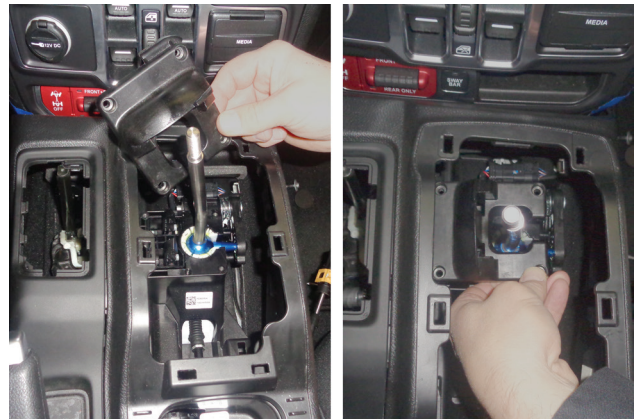
29. Set pivot cover plate (removed step 15) into position at base of shifter as shown.
