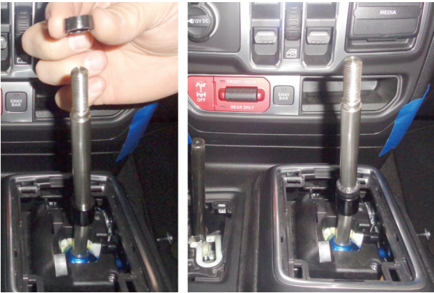
37. Install rubber stop (removed step 19) onto shifter assembly until it rests on lockout collar.
