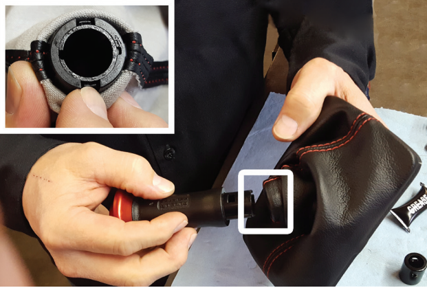
24. Remove factory reverse lockout top from boot by unclipping it at its base then pulling it out. Retain boot for next step.
