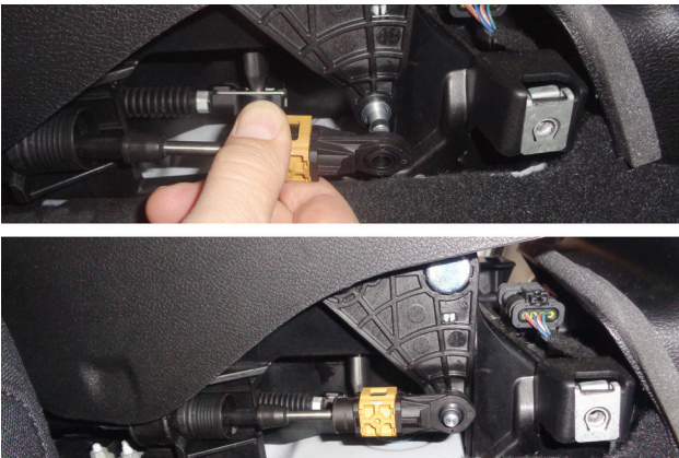
32. Install side cable onto side pivot arm, accessed from front passenger side of console.
