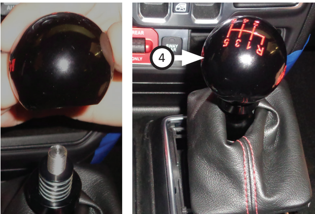
43. Install knob (4) onto shifter stem then finger-tighten it fully.
