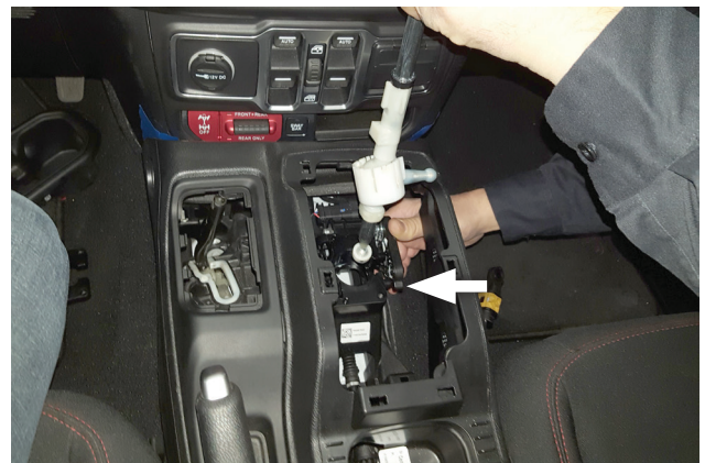
17. Lift shift lever upward while rotating side pivot arm upward to release shifter from base. Remove and retain shifter for later use.
