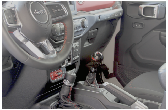
50. Ensure smooth and accurate engagement of all gears and proper operation of reverse lockout before starting car. Pay special attention to engagement of First, Second and Reverse gears.
