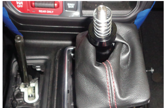
41. Place spring (removed step 5) onto shifter so it rests in reverse lockout.
