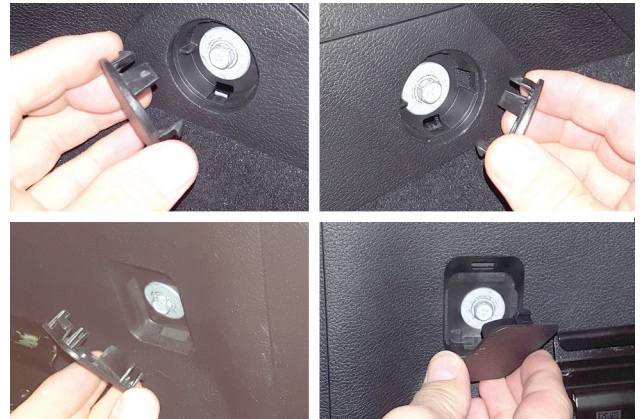
34. Install (x4 ea.) plastic caps and screws (removed step 13) into all four corners of console.
