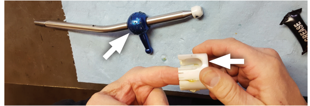
21. Apply grease from kit to pivot cup (removed step 20) and bottom pivot arm of shifter assembly (1) . Then install pivot cup onto shifter assembly.
