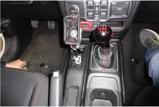
47. Place transfer case shifter (removed step 7) back into place on stem.
