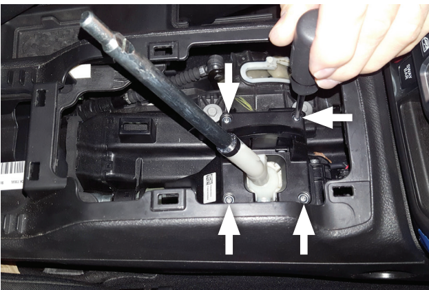
14. Remove screws (x4) and pivot cover plate from around base of shifter.
