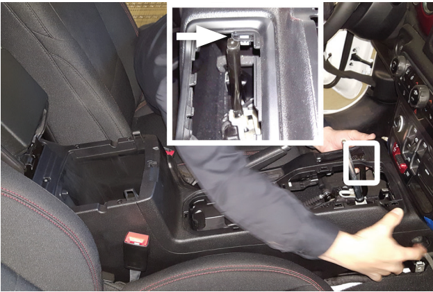
13. Pull up on front of console until you can use transfer case shifter stem as a prop for support.
