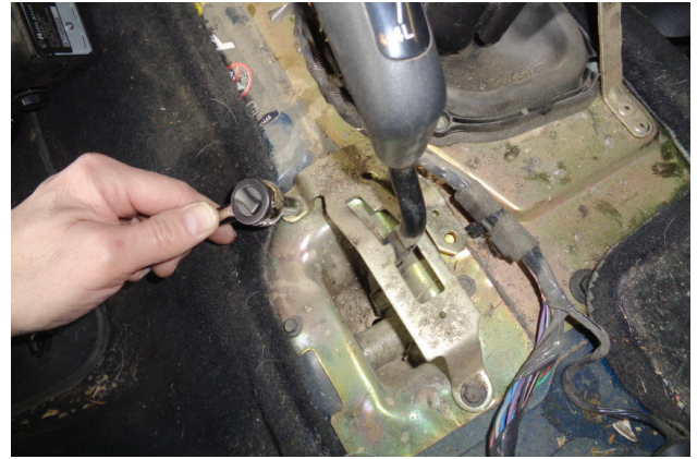
26. Reinstall transfer case shifter base.
