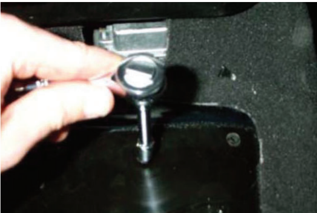
13. 1999-00 models: remove floor plate then proceed to step 17.
