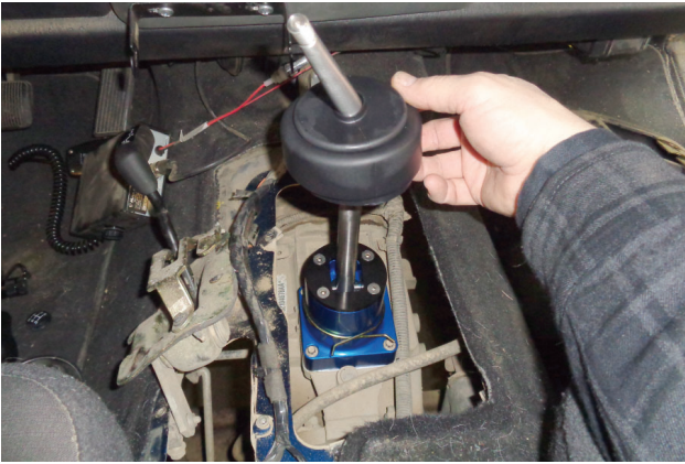
23. Install B&M dust boot over shift lever and shifter housing. Slide it fully onto housing, until inside of boot sits on top of housing.
