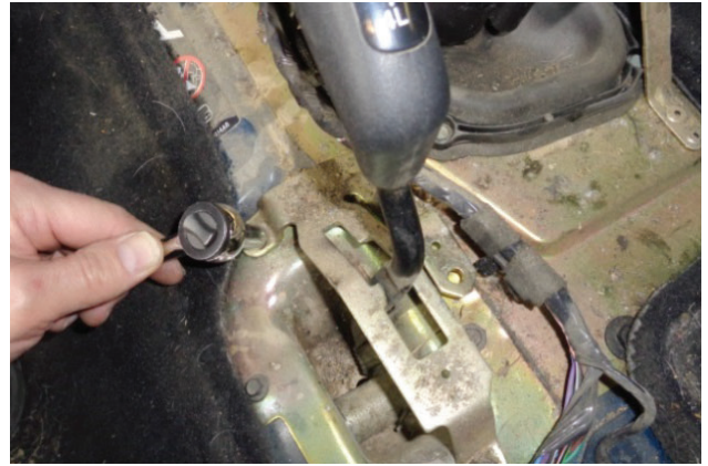
14. 2001-04 models: remove transfer case shifter base.
