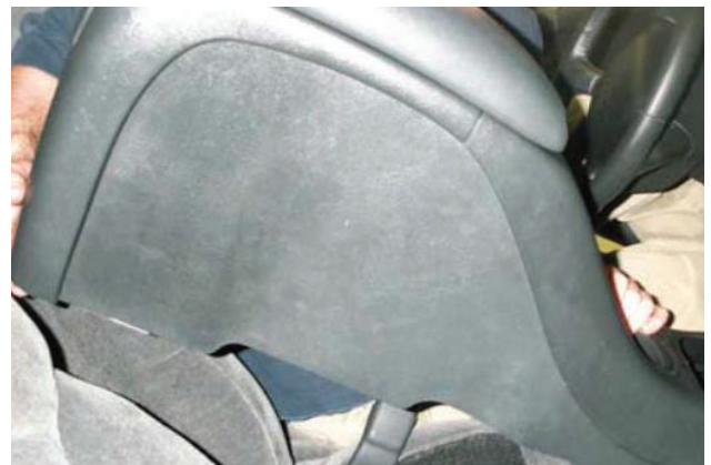
10. Engage parking brake lever for clearance, then remove entire center console (1999-2000), the front half of the console (2001-04), or the "mini" console (some 1999- 2004).
