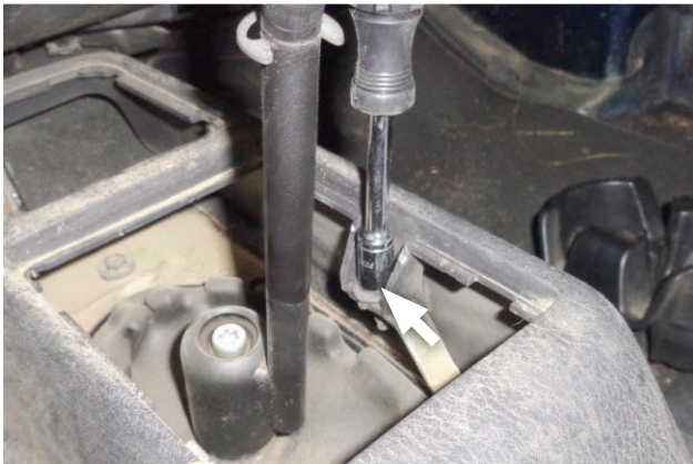
6. Remove center console bolt next to shifter.
