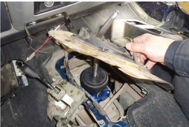
25. Reinstall floor plate.
