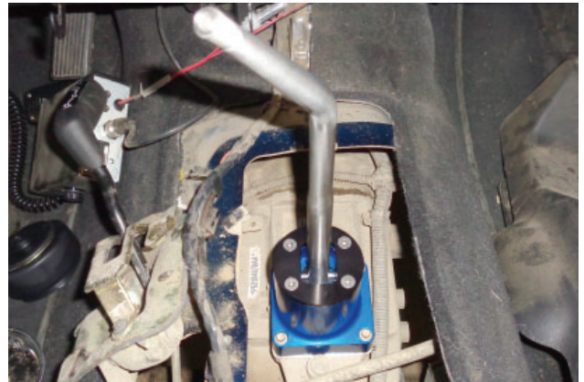
21. Install B&M shifter on transmission. Torque fasteners to manufacturer's specification.
