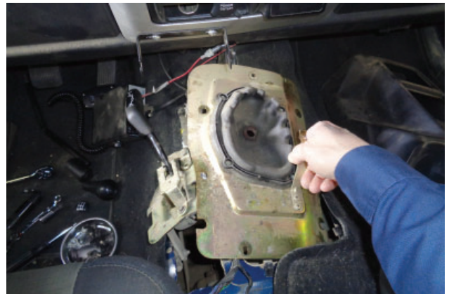
16. 2001-04 models: remove floor plate and attached dust boot.
