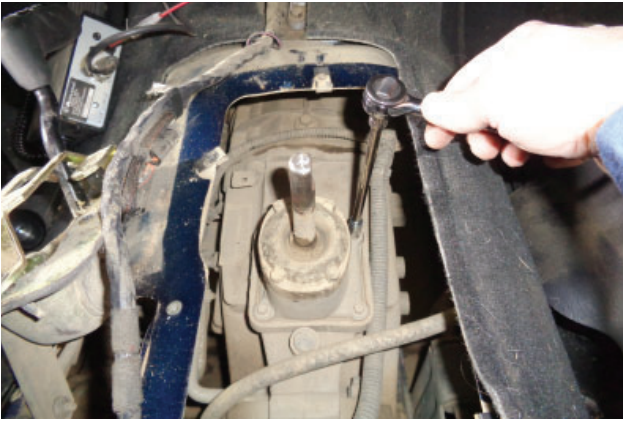
17. Remove stock shifter from transmission housing (4 screws at lower/square flange).
