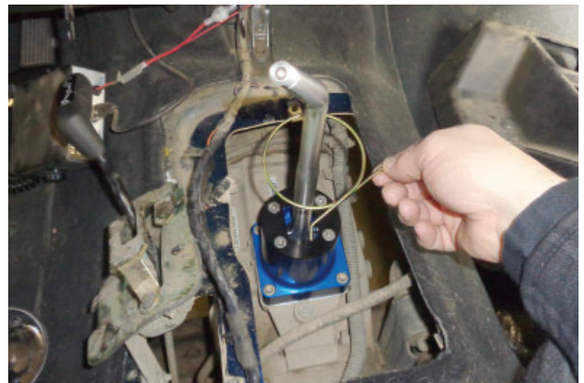
22. Place retaining ring over shifter and temporarily push it down to square mount flange.
