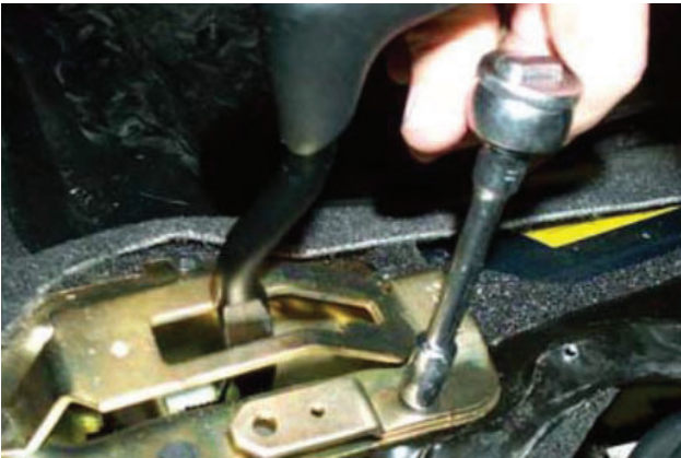
12. 1999-00 models: remove transfer case shifter base.
