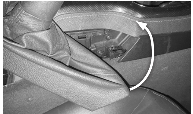
67. Reinstall the parking brake boot. First install the 2 plastic tabs on the right side of the boot, then reattach the 2 friction clips on the left side to the console base.
